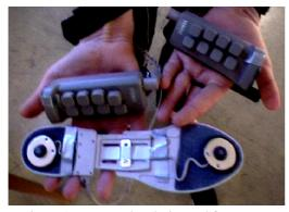
Figure 1. MIBURI handgrips and foot-sensor
